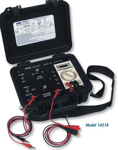
he ULTRA-TECH'S MODEL 14318 is a cut above anything in its class. This complete Portable Relay Tester comes fully operational and housed in a durable, lightweight, water resistant, and field-tested *railroad tough* carrying case. Our rugged, adjustable carry strap makes transporting the unit effortless. This model's proven track record insures that operating characteristics of vital signal relays meet OEM specifications while meeting Federal Regulations, under FRA Rule: 236.106.
